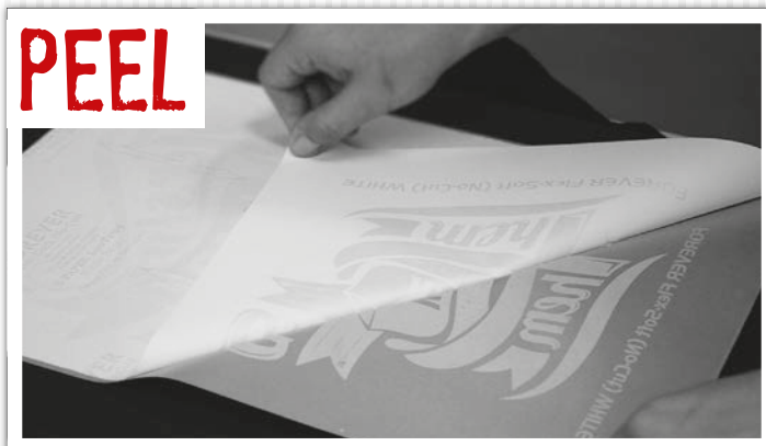
3 Peel A & B media apart and see, that the white opaque adhesive of the B-Paper LowTemp sticks only to the toner on the A-Foil. Now your transfer is ready.
