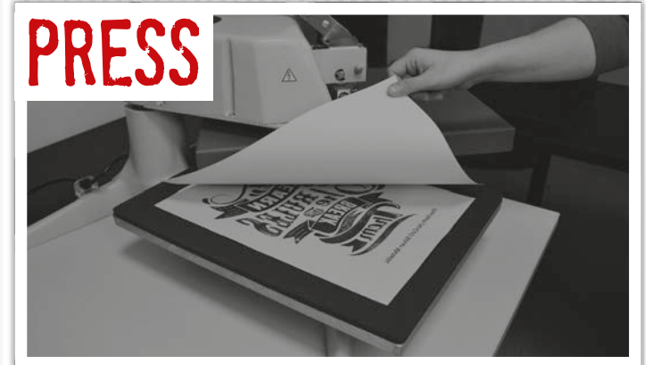
2 Press the A-Foil together with the B-Paper LowTemp
