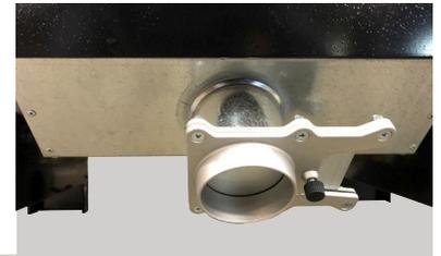
Exhaust Pipe with Adjustable Gate
