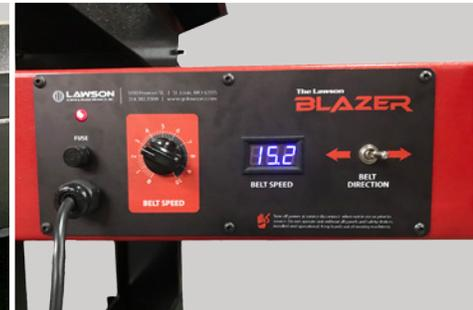
Digital Belt Speed Controls | Reversing Belt
